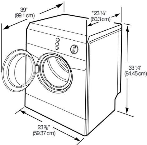
\*Most installations require a minimum 5 1/2" (14.0 cm) clearance behind the dryer for the exhaust vent with elbows. See "Venting Requirements."
