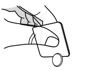
6. Depending on your model, remove the shoulder screw and its washer from the left-hand side of the door and fasten it into the hole that was behind the cap.
