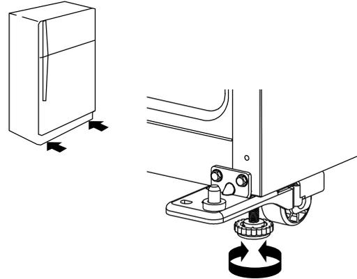
2. Open both doors again to make sure they close as easily as you like. If not, tilt the refrigerator slightly more to the rear by turning both leveling legs to the left; it may take several more turns.
